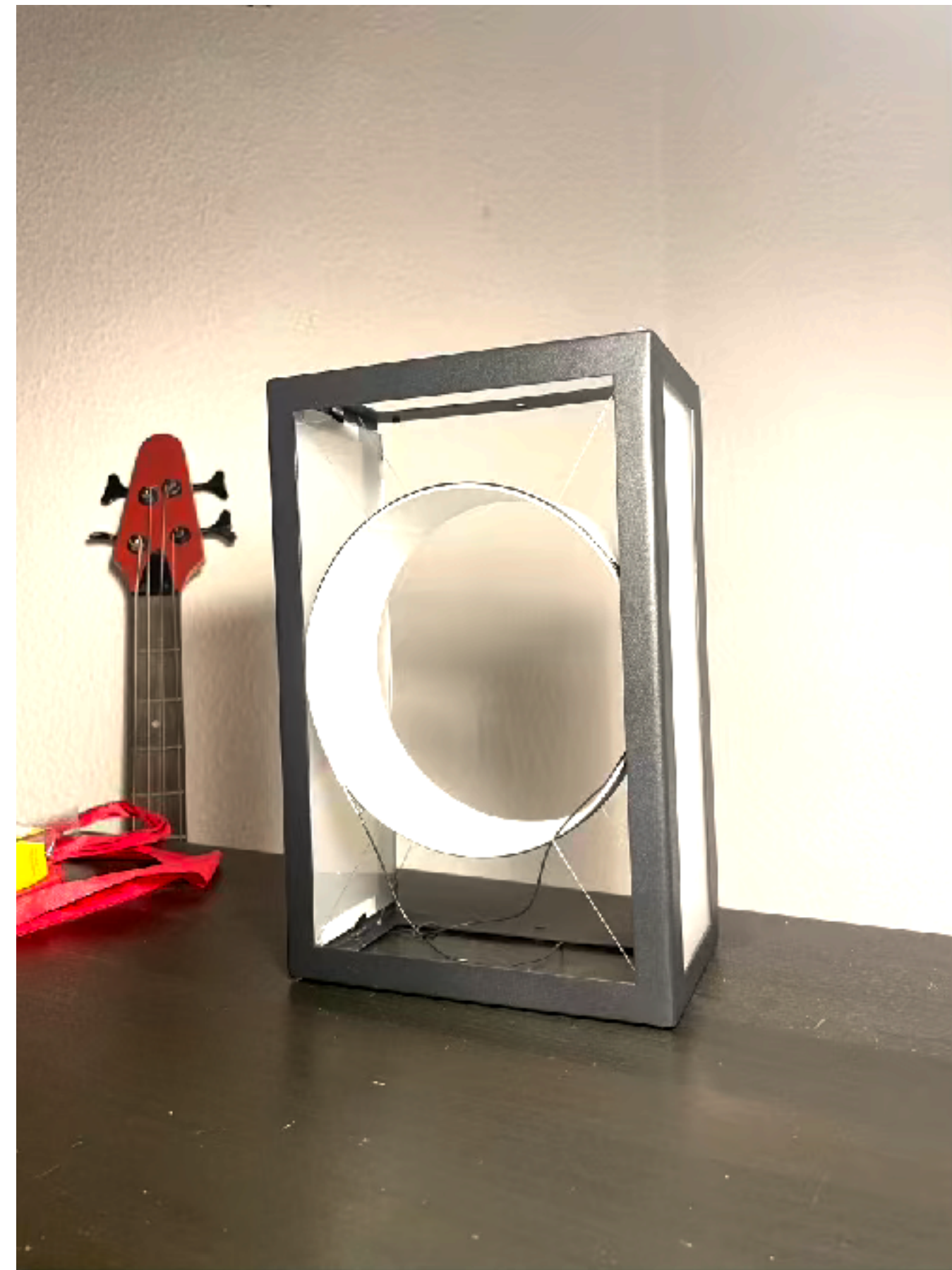
I drilled holes for nylon strings to hold the circular antenna.
